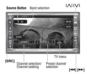
To switch Operation Screen ON, touch the center of touch panel or press [ENTER] on the remote control.
